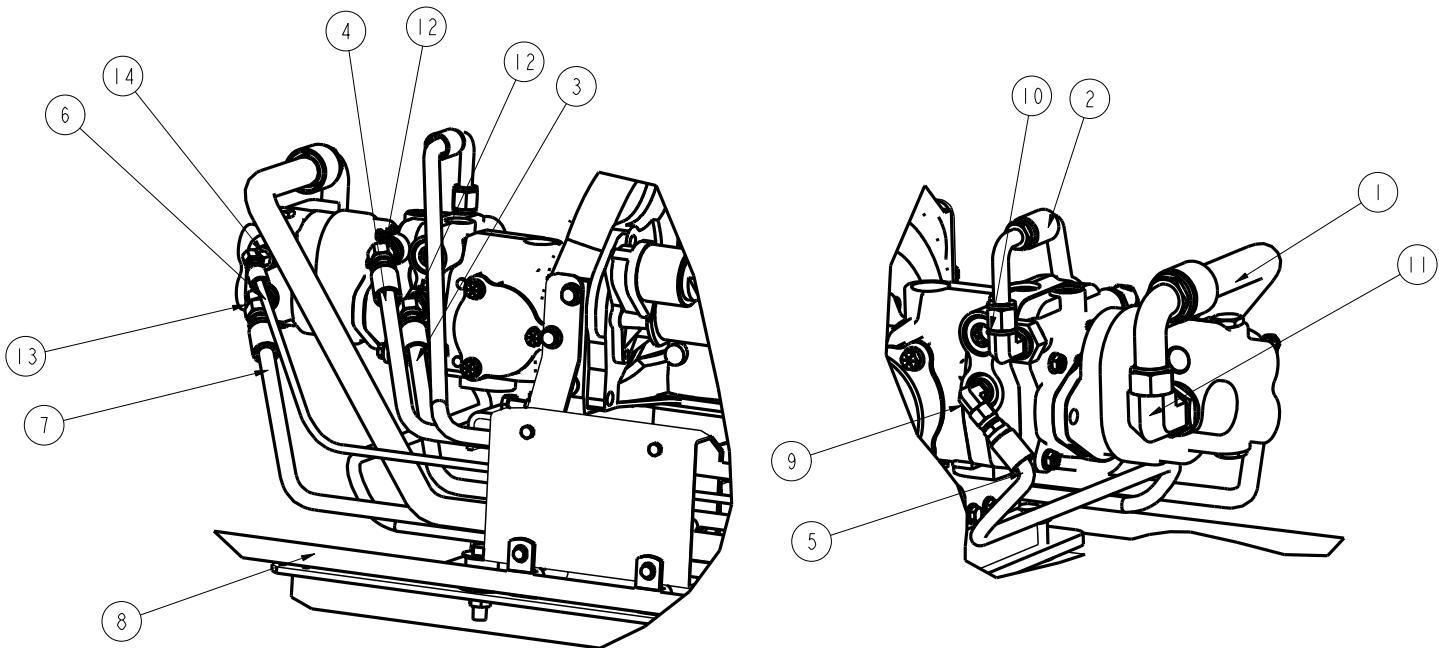
ENGINE GM 1.6L LPG & GASOLINE - HYDRAULIC HOSES & FITTINGS
