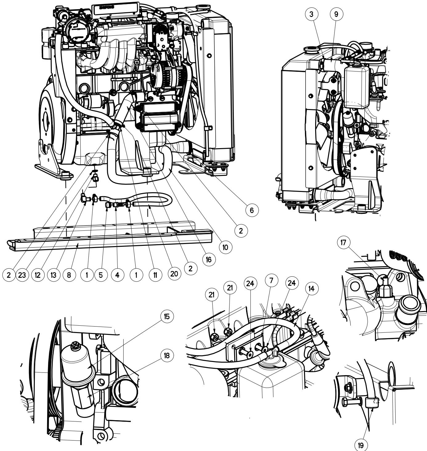
**ENGINE GM 1.6L LPG & GASOLINE - RADIATOR HOSES, SENDING UNITS & CLAMPS**
