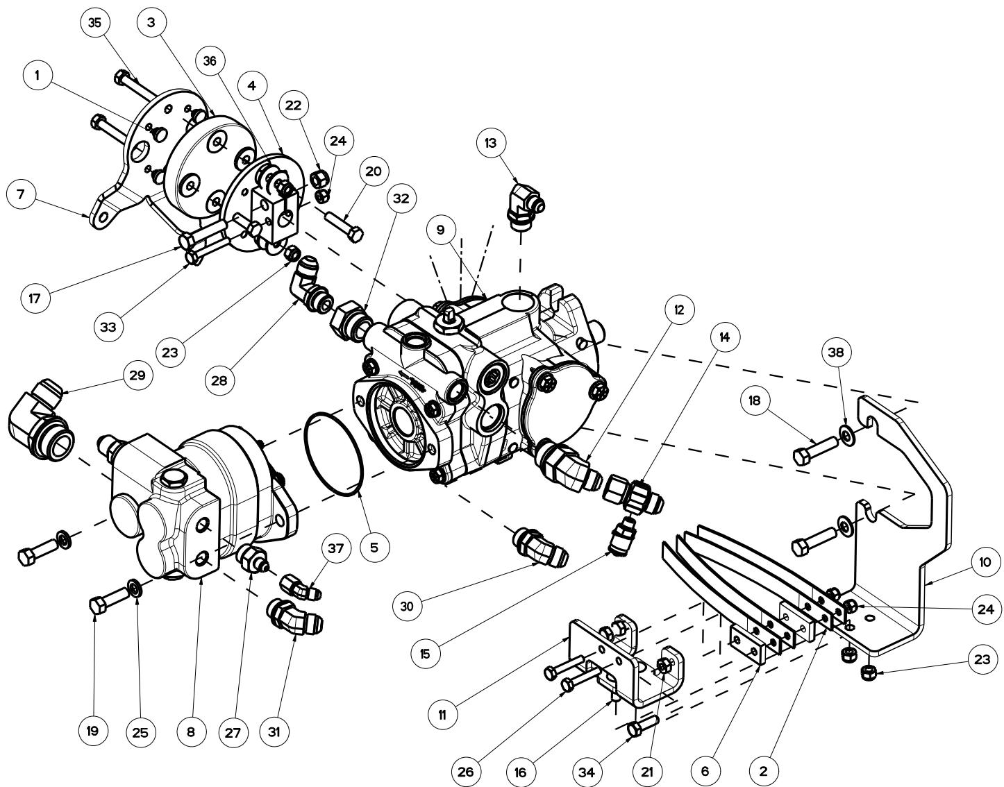
**2203 KUBOTA ENGINE - HYDRAULIC PUMP DETAIL**
