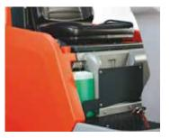
Adding the optimal amount of cleaning detergents in relation to the amount of water supplied in the cleaning process. The on-board dosing system is fully integrated into the machine.
