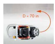
Can be used in narrow aisles and hallways thanks to its particularly compact design. 90 degree steering angle, turning circle of only 70 inches.
