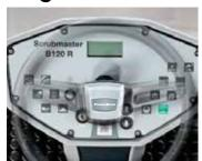
Illuminated, intuitive display: with a 1- button operating system, boost button for maximum water supply and brush pressure, and slow mode activation -- all at the push of a button.
