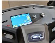
Illuminated and intuitive display: Indicates the battery charging level and the filling level of the solution and recovery tank.
